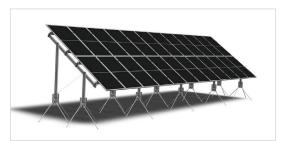
3 mm thickness of the "legs" 2 mm thickness of transverses 1.5 mm thickness of longitudinal The calculation was carried out with the following loads: snow load up to 1.6 kN/m2, wind up to 24 m/s
